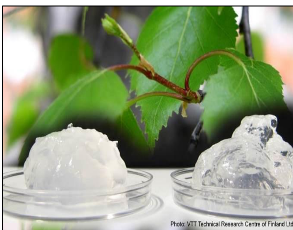
Adhesive-free consolidation treatments using Nanocellulose Gels
