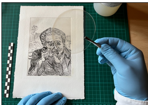
Making of highly transparent Nanopapers for mending treatments
